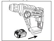
To remove the battery pack, slide it from the tool while sliding the button on the front of the cartridge.
