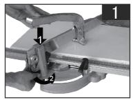
1.Before operating, adjust the adjusting screw to make the height of handle in perfect position to cut the tile easily. (figure 1)
