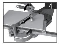
4.After locating, lift the handle, make the cutting wheel on the tile, and cut the tile slowly. (Figure 4)
