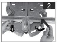
2.Press down the locating screw to zero graduation line, make it and pointer of swivel overlaping. Then tighten the clamp handle, make scaleplate and pressure line overlaping. (Figure 2)
