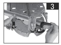
3.Press down the locating screw to make it locate in any degrees from 0 to 45°. Then tighten the clamp handle. (Figure 3)
