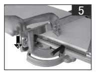
5.After cutting, put handle near the end face of the tile,then push down, making the tile break. (Figure 5)
