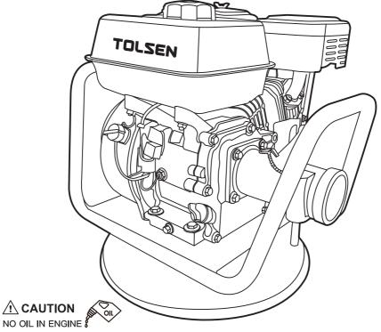
Fill the engine with oil to the correct level before starting the engine.
